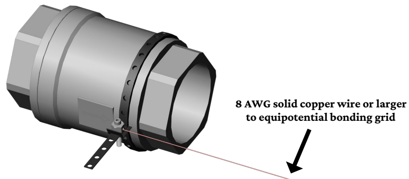
Check Valve with a Bonding Clamp
